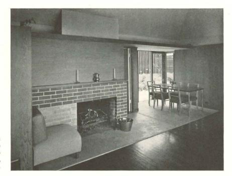
Omission of a partition between living room and dining alcove adds to the spaciousness of the area. Walls are redwood plywood, untreated; hearth is concrete.
