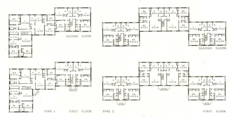
The Parklane Apartments are of brick-veneer construction with specially constructed steel frame and concrete floor slabs. The frame is sheathed with sheathing wallboard and faced with rusty-pink brick and warm gray-white stucco. Fenestration consists of both steel casements and glass-block panels. The roof is of galvanized iron, 29 gauge, with standing seams and covered with four-coat asphalt and sand treatment with a white cement-base finish coat.
