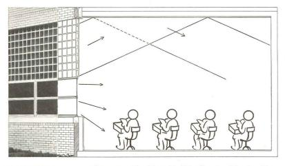
**BETTER LIGHT** for every pupil in rooms like this, with light-directional Insulux Glass Block above steel sash. The block throw light to ceiling, which reflects it evenly over room. Light-directional block are used on any exposure without objectionable glare.
