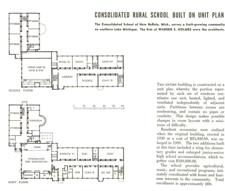
The entire building is constructed on a unit plan whereby the portion represented by each set of windows constitutes one unit, heated, lighted, and ventilated independently of adjacent units. Partitions between rooms are nonbearing, and contain no pipes or conduits. This design makes possible changes in room layouts with a mini-
