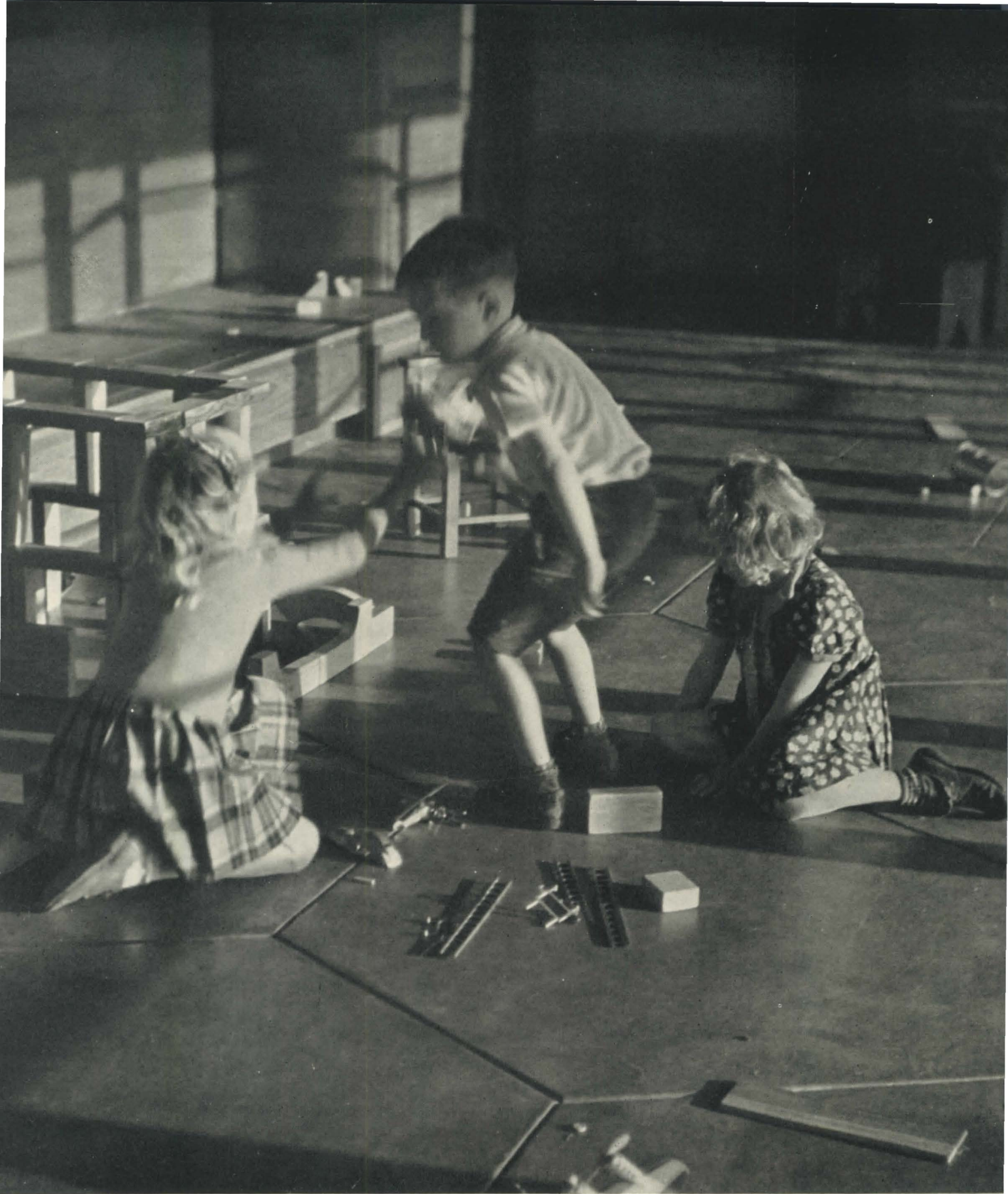
This nursery playroom has an easily cleaned cement floor which is heated in winter. Frank Lloyd Wright was the Architect.
