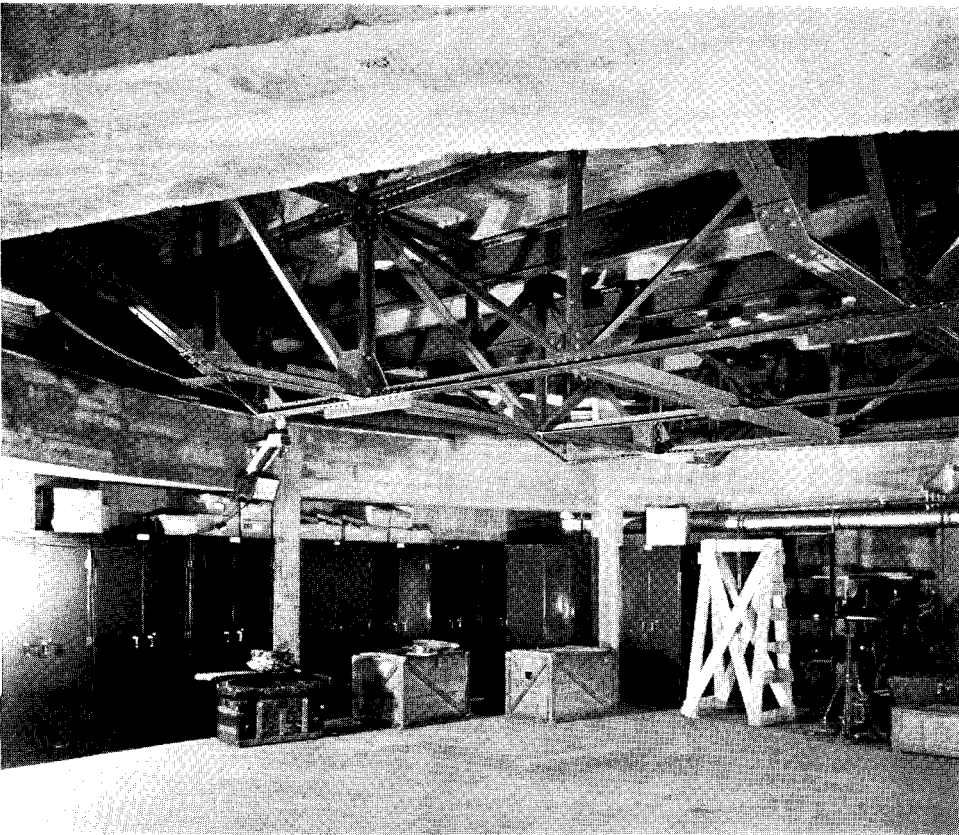
Below the revolving stage, clear trap-space is left.
