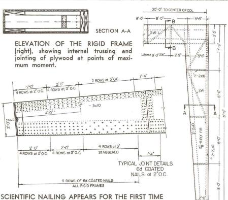
in these lumber and plywood rigid frames. Since fabrication on the site eliminated controlled gluing, the nailing had to be as carefully analyzed as riveting in steel.
