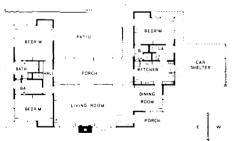
Living room, dining room and porch are so arranged that they can form one large living space, with a free passage of air. Further ventilation is obtained by screened louvers between the roof sheathing and the room ceiling, thus helping to avoid the usual intense heat from flat roofs. The car shelter also has louvers which exclude the sun, and ventilate at the same time.
