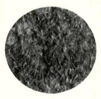
"Armco Galvanized Paintgrip" (40 diameter microphotographs)
