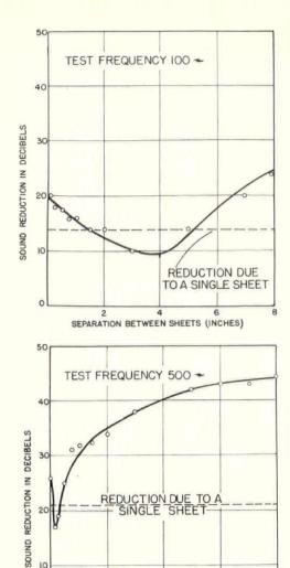
The sound insulation values are given in terms of the decibel. For example, a window which transmits I/I0th of the sound which falls on it has a sound insulation of 10 decibels; if it transmits I/I00th, 20 decibels; I/I000th, 30 decibels, and so on.
