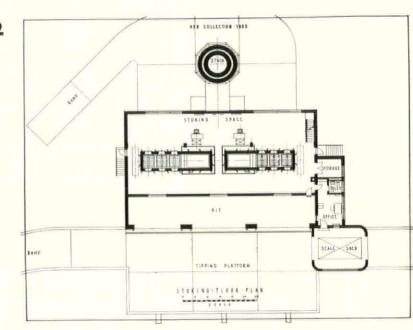
Refuse, brought by truck to the tipping platform (2) is dumped into the pit. Traveling cranes pick it up and dump it through hoppers (3) into the furnace chamber. The ash is then dropped into trucks on the basement level (1) where it is hauled out.
