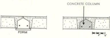
columns are cast in place at juncture of wall units
