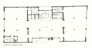
with a pumice screed, 3 to 4 inches deep above to make up the levels and allow pipe ducts to be formed. The ceilings were plastered on suspended metal lathing the space between the structural slab and the lathing permitting easy allocation of sprinkler pipes and point. In most cases the depth of the floor from finished level to underside of plaster work is about 1 foot 9½ inche. On the ground floor, travertine slabs 2 feet by 2 feeby 1 inch thick have been used throughout as a part
