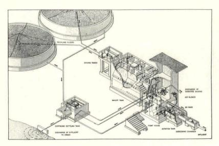
The design of the disposal plant is based on a pro-rated fa of 3.8 persons per house and an ultimate population of 5, gi a total of 1,000; and providing for a wet water flow of 100 gal of water per capita daily. The plant consists of the following u Bar Screen, Aeration and Skimming Tank, Imhoff Tank, Tricl Filters, Dortmund and Chlorination Tanks, with a discharge in stream affording an average dilution of approximately 10 ga of water to one of sewage effluent.
