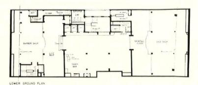
are divided by 13½-inch brick walls and double fire shutters to the openings from one block to the other, the opening consisting of a 10-foot one on the main axis of the building and a 24-foot opening, one either side of the central space.
