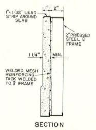
section of Haco stone slab measuring 3'-4'' wide and 5' high
