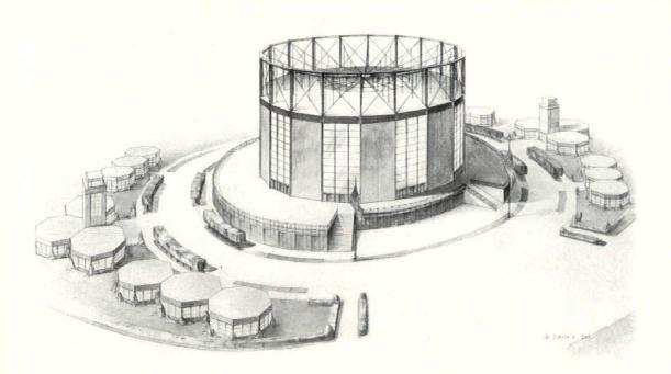
Proposed design for an exposition building at the 1939 World's Fair in New York, utilizing a self-anchored steel suspension system. Simon Breines, architect. Robinson and Steinman, consulting engineers.
