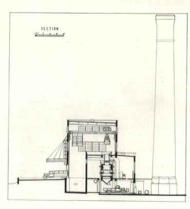
Cross section of plant showing relation between refuse deposited by truck (lower left) to ash removed by truck (lower right).
