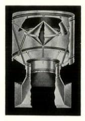
roof ventilator without moving parts
