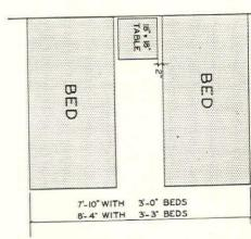
BED WIDTHS AND REQUIRED SPACING OF TWIN BEDS.
