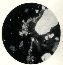
figure 4 — well-defined layer and intimate bond occur when lime is added and brick has reasonable absorption
