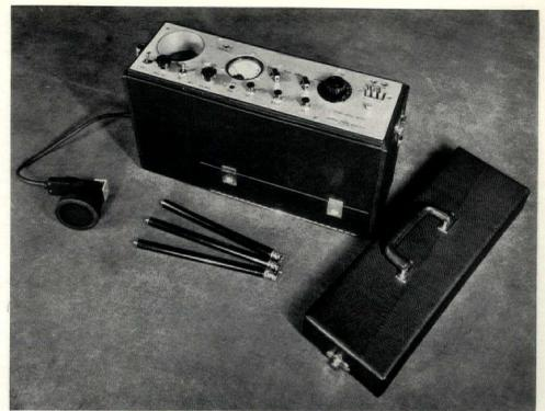
sound level meter used in measuring conditions of noise
