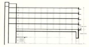
SECTION SHOWING PRESENT STRUCTURE WITH PROPOSED ADDITIONS
