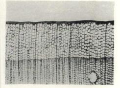
a definite line marks extent of controlled oil penetration in a new type of paint
