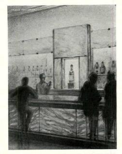
SKETCH BY VAHAN HAGOPIAN FOR AN INTERIOR OF A BAR. Lumar is used here: A. For general illumination as a translucent shade for a continuous wall bracket. The light is allowed to escape freely and illuminate the walls which, in turn, indirectly light the room. B. Lumar is used decoratively only as a front to the bar itself, taking advantage of its translucent qualities.
