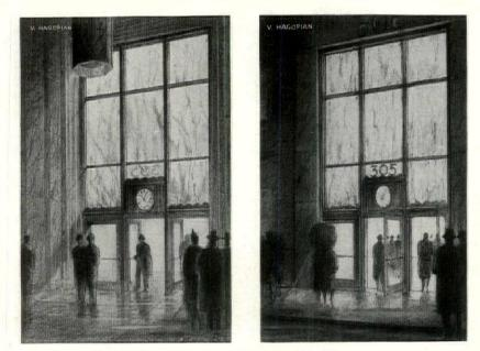
SKETCHES BY VAHAN HAGOPIAN FOR THE USE OF LUMAR IN INCLOSING THE OPENING ABOVE THE DOORS OF AN ENTRANCE LOBBY. LEFT: A view of the interior of the lobby illuminated by natural daylight through Lumar. RIGHT: The exterior by night when the translucent properties of Lumar transmit the artificial light of the interior and thus add to the decoration of the building.
