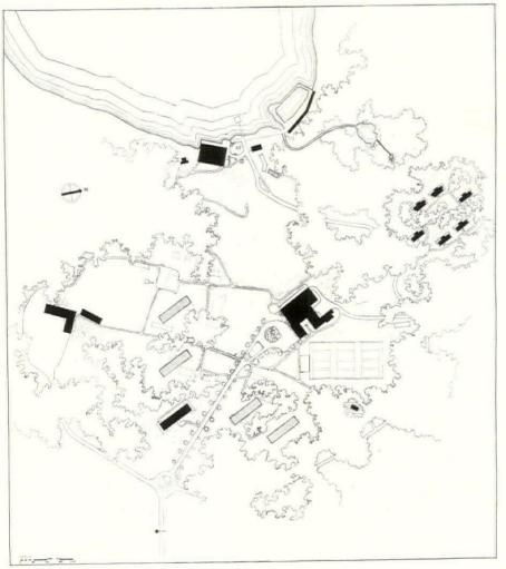
**Plot Plan:** Structures in solid block to remain in finished development; gray indicates structures planned, dotted lines those to be wrecked The new buildings are all oriented to take fur advantage of view and exposure. The resort has two handball courts, nine tennis courts, two bass ketball courts. Water sports of all types ar provided for in the large lake on the premises
