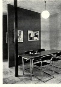
DINING ALCOVE IN LIVING ROOM. tition produced by simplest means, nar 1" plywood with lumber core.
