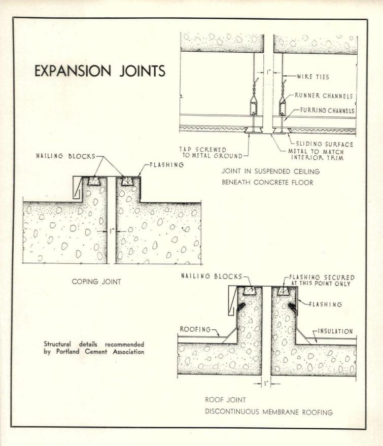
or the like, joints at one or both ends of the vulnerable section may be in order. Where a building changes direction, as in L-, T-, or U-shaped plans, joints are generally advisable. Suggested expansion joints are shown in the accompanying illustrations.
