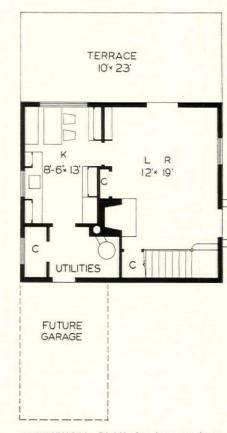
ECONOMICAL PLAN for low-cost house Frank J. Forster, architect. Plan of squ shape, dining alcove in kitchen, and din space in living room, kitchen combined v utility room. Exterior walls 8" cinder b and double core furring. Floor framing, cast concrete joists and cinder slab filling v wood floor finish. Total cubage, 8,705 c feet.
