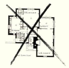
HOUSE FOR DEVELOPMENT. Costly because of broken contour of house plan. Lack of simplification of floor arrangement.
