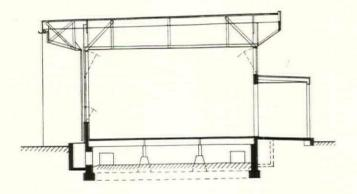
CROSS SECTION, SHOWING EARTHQUAKE-PROOF CONSTRUCTION
