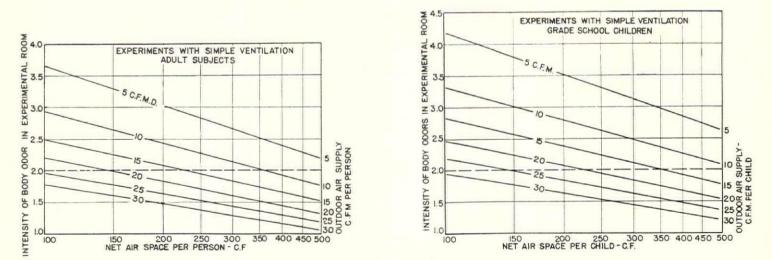
charts for computing ventilation requirements from standpoint of body odor: for example, given an air space of 300 cubic feet for each person, follow vertical line indicating this condition until it intersects the broken horizontal line representing the allowable odor intensity of 2; by interpolation the required outdoor air supply is found to be 12 cfm for each adult, 17 cfm for each child.
