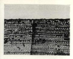
microscopic view of cross-section of wood shows penetration of ordinary paint oil
