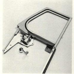
automobile window regulating mechanism
