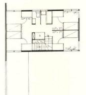
PLAN. SECOND FLOOR. All wardrobes standard, namely, id cal in size and forming part of partitions. Bath and toilet separa making for double capacity of single bathroom.
