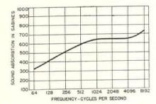
desired sound absorption for acoustic materials in a studio of the size indicated by the plan shown above
