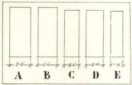
DOOR WIDTHS RECOMMENDED BY PWA (HOUSING DIVISION). (a) ENTRANCE, (b) BEDROOM, (c) BATHROOM, (d) CLOSET, (e) LINEN CLOSET. DOOR HEIGHTS, 6'-4", 6'-6", 6'8"; CLOSET DOORS MAY BE 6'-2" HIGH.
