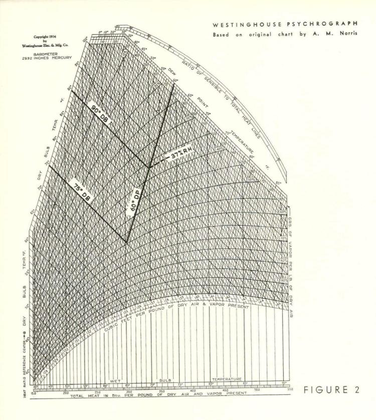
Given: Dew-point temperature 60° and dry bulb 75°. Find: The relative humidity, should the dry bulb be increased to 90° with no moisture added (dew point remaining constant).
