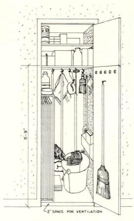
CLEANING CLOSET (SIZE, 14" x 27" OR 17" x 25"). DIMENSIONS AND ARRANGEMENT BASED ON EQUIPMENT AND SUPPLIES FOUND IN REPRESENTATIVE HOME OR APARTMENT. 5 HOOKS FOR LONG ARTICLES; 4 HOOKS FOR SHORT ARTICLES. UPPER SHELF 9" DEEP; LOWER SHELF 14" DEEP. DESIGNED BY MAUD M. WILSON, HOME ECONOMIST.
