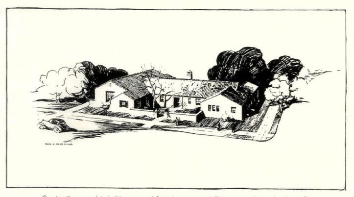
Construction completed this year; reinforced concrete walls, cement plastered; tile roof.
