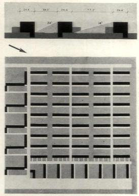
DIAGRAM OF HOUSING OF MINIMUM AND MAXIMUM DESIRED SPACING. ORIENTATION PERMITS FULLEST EXPOSURE TO EAST, SOUTH AND WEST. FOOTPATHS PARALLEL BUILDINGS. THERE IS NO MAIN TRAFFIC CROSSING THE HOUSING AREA.
