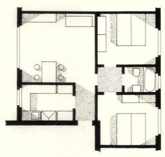
(4) INTERIOR AND DAYLIGHT. WINDOWS WITH DESIRABLE RELATION TO ROOMS, PARTITIONS AND FURNITURE. CONSIDER DESIRABLE DAYLIGHT ON WORK SURFACES AND GOOD VISION FOR ALL PARTS OF A ROOM FOR BOTH CLEANLINESS AND TO FAVOR A GENERAL IMPRESSION OF CHEERFULNESS.
