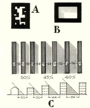
(A, B AND C) COMPARISON OF OLD AND NEW METHODS OF BLOCK DIVISION. (C) RELATIVE COVERAGES AND SUNLIGHT EXPOSURE FOR TWO-, THREE- AND FOUR-STORY DWELLINGS. SPACING IS INDICATED FOR DWELLINGS FACING SOUTH IN ORDER TO PROVIDE FULL SUNLIGHT AT 45 DEGREES. H. WRIGHT.
