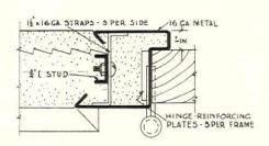
SOLID 2" PLASTER PARTITIONS. 3/4" CHANNELS SET 16" O. C. INTO CHANNELS AT FLOOR AND CEILING. DOOR FRAME OF 16-GAUGE STEEL. TECHWOOD HOUSING PROJECT AT ATLANTA, GEORGIA.
