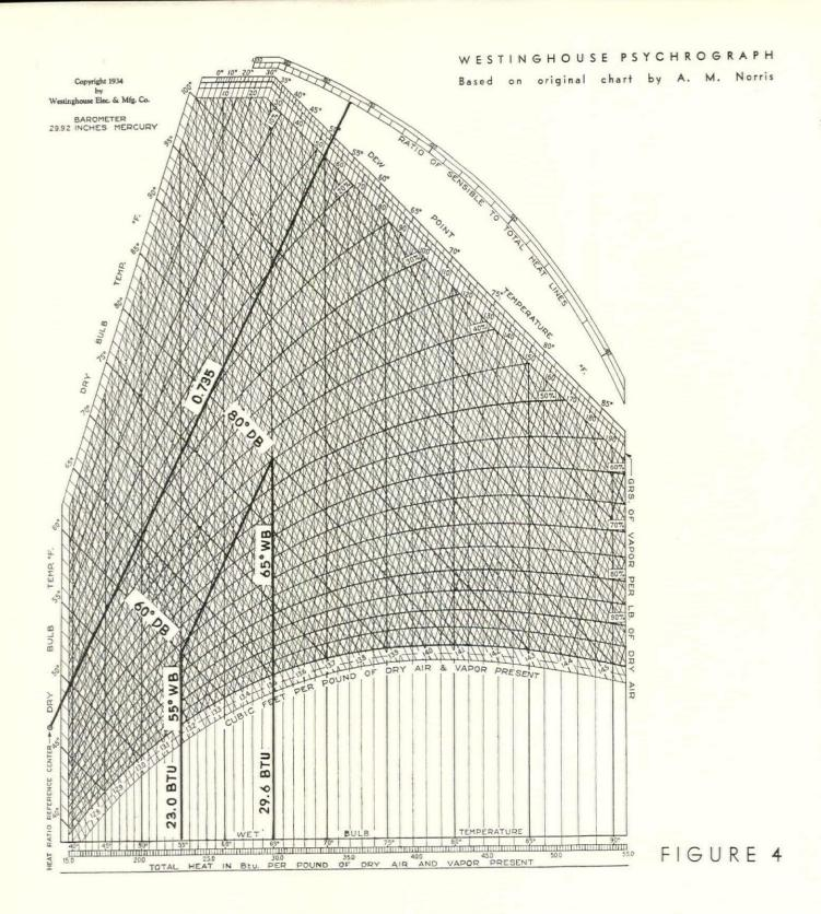
Given: Air cooled from 80° dry bulb temperature and 65° wet bulb temperature (about 45% relative humidity) to 60° dry bulb temperature and 55° wet bulb (72.5% relative humidity).
