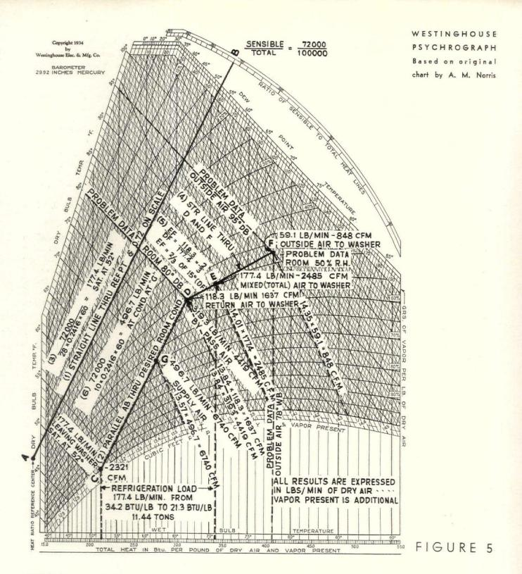
This figure illustrates a graphic solution of an air conditioning problem in which it has been assumed that a by-pass system, using a washer, will be installed.
