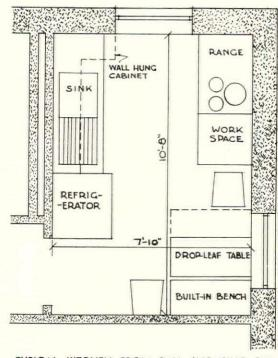
TYPICAL KITCHEN FROM PWA (HOUSING DIVISION) "SAMPLE PLANS." THERE IS DESIRABLE CROSS CIRCULATION OF AIR; DINING TABLE, WITH DROP LEAF AT WINDOW.
