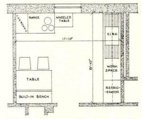
KITCHEN WITH WORK AREAS AT RIGHT-ANGLE WALLS; CUPBOARD FOR KETTLES AT SIDE OF RANGE; DINING TABLE AT MOST CONVENIENT LOCATION.
