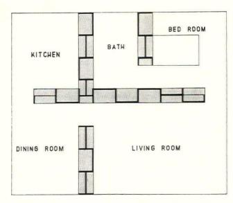
FLOOR PLAN IN WHICH ROOMS ARE SUBDIVIDED BY CLOSETS AND CABINETS OF STANDARD SIZE, INSTEAD OF BY PARTITIONS. SUCH AN ARRANGEMENT CAN BE ECO-NOMICAL TO CONSTRUCT AND CAN GIVE UNITY OF APPEARANCE TO ROOMS. THE ARRANGEMENT OF ROOMS CAN BE READILY CHANGED.
