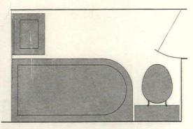
BATHROOM OF NARROW ARRANGEMENT WITH ACCESS FROM HALL; 311/2 SQUARE FEET. BATH-ROOM SIZE 4'-11" x 6'-8" (33.2 SQUARE FEET) SUITED TO "SAMPLE PLANS" ILLUSTRATED IN THIS
