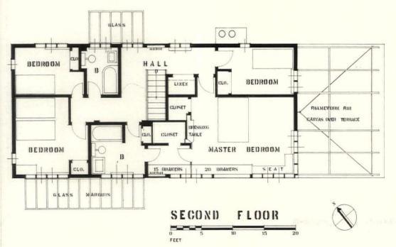
The owner's bedroom, dressing room and bath are of comfortable size and provide ample facilities, while the other bedrooms and bath are held to rigidly minimum dimensions. The positioning of bathrooms and kitchen centralizes all plumbing, reducing the cost and minimizing the damage from possible pipe failure. Copper water tubing is used throughout.
