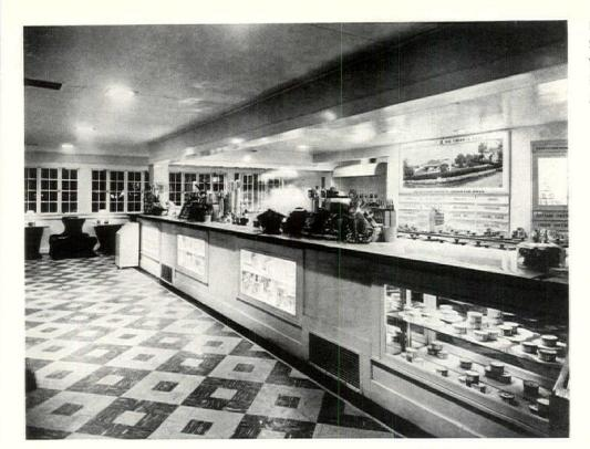
LIGHT IN THIS ROADSIDE STAND IS DIRECTED DOWN-WARD FROM FLUSH CEILING PARTS ON TO THE SERVICE AND TABLE AREAS.
