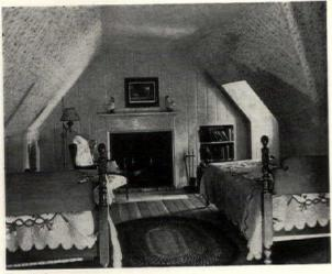
ATTIC SPACE USED FOR BEDROOM. INSULATION SHOULD BE APPLIED TO WALLS AND CEILING. CROSS VENTILATION IS PROVIDED BY WINDOWS ON OPPOSITE WALLS.
