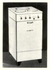
\*NEW TYPE ELECTRIC FLUSH TOP RANGE, 18" WIDE, 24" DEEP, 36" HIGH. COOKING UNITS: TWO 61/2" DIAMETER, 1,000 WATTS: ONE 81/2" DIAMETER, 2,000 WATTS. OVEN UNIT: 14" WIDE, 18" DEEP, 18" HIGH, 3,000 WATTS. PRICE AT THE FACTORY, \$72.
