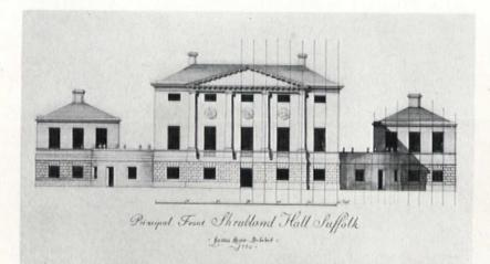
Drawings accompanying this article demonstrate the exactness with which similar dimensions are repeated. The design formulas of classical antiquity were based on order. Vitruvius, Vignola and Palladio codified the principles of a module system.
