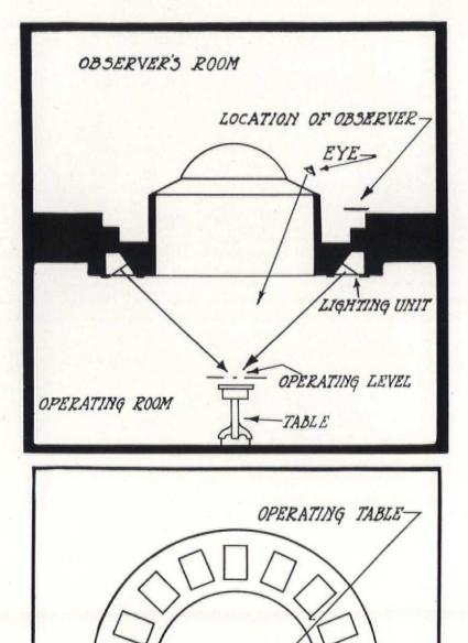
A circle of Holophane lighting units set flush in the ceiling under the observation gallery is of a diameter which places the light sources in the dead space between the patient's and the surgeon's normal fields of view. The position of the lights likewise does not interfere with the vision of the observers.
