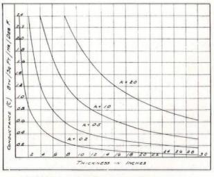
FIGURE I: EFFECT OF INCREASE IN THICKNESS ON THERMAL CONDUCTANCE
