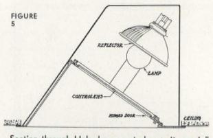
Section through Holophane controlens unit, specially designed to concentrate a series of high intensity, superimposed beams on the operating area.
