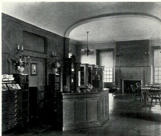
Hart Free Library at Townsend, Mass. The trim is of stained oak, with rough plaster above. The floor is of cork tile and the cornice is plaster. All furniture in the children's room is of small sizes. The light fixtures are dark bronze.
