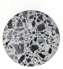
Cross section of Featherweight Concrete, slightly enlarged, showing the cellular nature of the Haydite aggregate and the dense, impervious structure of the concrete.
