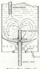
Arrows show action of Arrows show action or water when drawn thru TURBO-AQUATHERM scouring bottom of boiler and preventing any ac-cumulation of sediment
