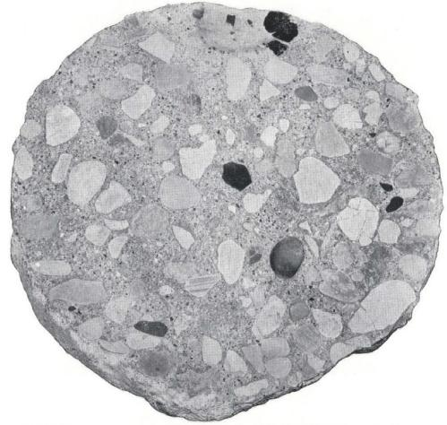
$\mathbf{G}^{\text{OOD}}$  concrete, compressed by the MacARTHUR method, insures piles of greater bearing capacity. The rough concrete is intimately bonded with surrounding soil.
