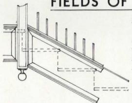
HE new J & L 12" Light Weight Steel Channel embodies all the savings in weight and time required for fabrication and installation which have made the 10" section so popular in stair construction, and extends the field in which those advantages may be applied.
