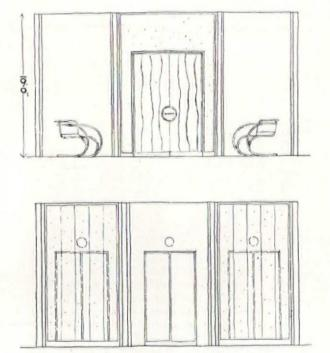
Walls of the reception room are of colored transparent glass. The wall between library and reception room is of opaque glass. The glass is held in place by aluminum-plated steel columns. Floor in black and gray linoleum. Illumination from PH lighting fixture. Chairs and tables are of MR (Mies van der Rohe) design.
