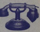
Connecticut Cradle Phone is new in design and equipped with bakelite hand phone. Supplied complete with 6 foot mercerized cord and terminal block. May be substituted for conventional desk type phone. Removing hand phone connects the instrument to the talking circuit. Is furnished with 4 6 or 8 hutters. Physical with 4, 6, dull black. 6, or 8 buttons. Finish is
