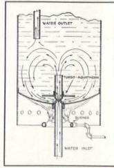
Arrows show action of water when drawn through TURBO-AQUATHERM, scouring bottom of boiler and preventing any accumulation of sediment.
