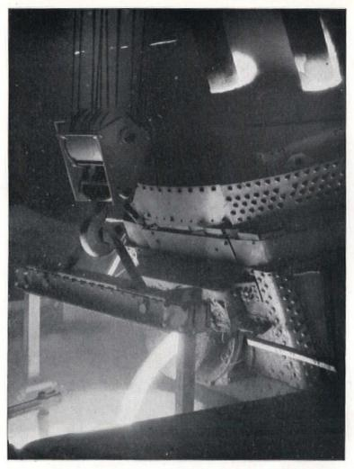
Tapping a twenty-five ton Electric Furnace in one of the two modern plants in which Republic produces Enduro Nirosta KA2, the perfected Stainless Steel—under the original Krupp patents.
