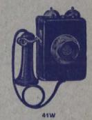
Connecticut Surface Wall Telephone has hinged metal case, standard trans-mitter and receiver, double gong bell, and one button for calling central, All outgoing wiring in hinged front is cabled to terminals on face of back. Terminal screws threaded into brass bushings. Back drilled fir single-gang outlet box mounting. Finished in baked black enamel.
