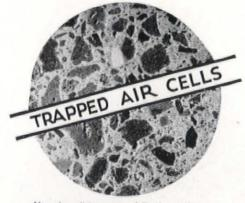
Note the cellular nature of Featherweight concrete which makes it light and insulating, yet with concrete's standard strength and density.
