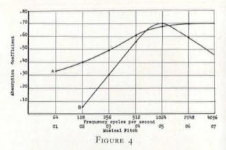
COMPARISON OF THE ABSORPTION FREQUENCY CHARACTERISTICS OF TWO COMMERCIAL SOUND ABSORBING MATERIALS
