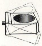
This is the exclusive NORWALK Self-Adjustable Strike that engages bolt from any angle and locks the door regardless of shrinkage, warp or sag.
