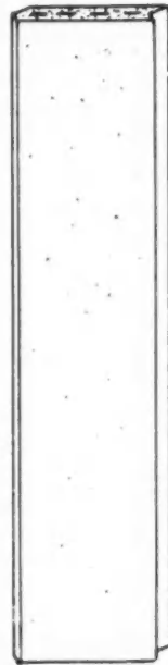
TEKTON INSULATING BLDG UNITS WOOD SHAVINGS WITH MAGNES- ITE CEMENT & REINFORCING WOOD STRIPS 11'-6" LONG
