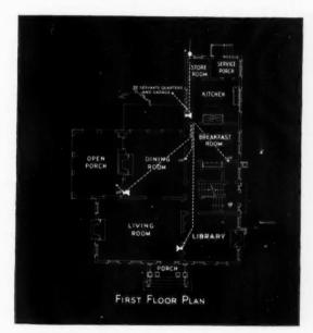
In the residence of Mr. J. W. Goldsmith, of Atlanta, three telephone outlets downstairs and six upstairs provide facilities for installing telephones at convenient locations. There is an additional outlet in the servants' quarters over the garage. Exposed wiring is made unnecessary by the conduit layout. PRINGLE AND SMITH, Architects.
