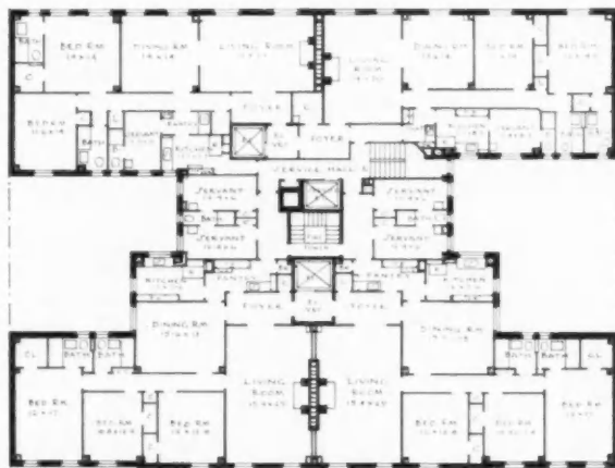
FIG. 17. PLAN OF TYPICAL FLOOR ARRANGEMENT: FOUR APARTMENTS—2 OF EIGHT AND 2 OF FOUR ROOMS
