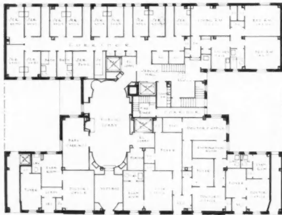
FIG. 15. PLAN OF STREET OR ENTRANCE FLOOR, DOCTORS' OFFICES, SERVANTS' ROOMS AND SUPERINTENDENT'S APARTMENT
