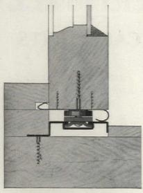
Half size section showing New Spring Track with Sliding Shoe attached, also Arm and Window Attachments with Double Spring Action Weathering Member.
