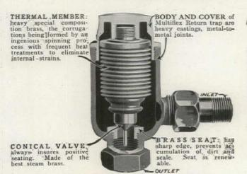
THE B & B Multiflex Return Trap is radically different from others and a decided improvement in many respects. Condensation discharges rapidly, owing to the immediate response of valve to slightest change of temperature. This trap with its pleasing outlines is not objectionable to the most exquisite furnishings.
