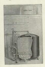
Sectional View of Refinite Water Softener
