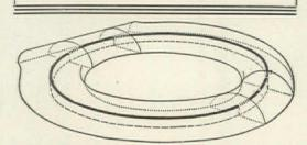
This sketch shows the method of construction of the "Allright" Seat with the steel hoop in place.
