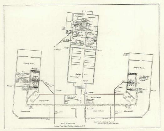
FIG. 3. PLUMBING LAYOUT FOR DORMITORY WITH KITCHEN AND MESS HALL ANNEX.
