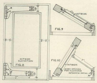
This Hinge overcomes the one objection to the otherwise popular Out-Swinging Casement Sash, in that it permits the sash to be swung around so that the outside of the glass can be cleaned from the inside. Hinge No. 90 For Outswinging Casement Sash
