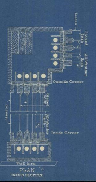
All-Weather Sash in Use Main Sill -Outs Sill Wainscoting Glazed Sash in Pocket When not in Base Finish Floor Rough Floor Joists
