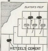
Hetzel's E. R. R. Cement prevents slates from loosening or falling out when nails or hooks rust off.
