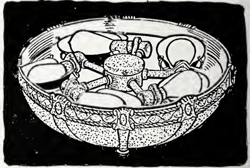
Fig. 3. Top view of the fixture illustrated in Fig. 2, showing arrangement of lamps and reflectors.
