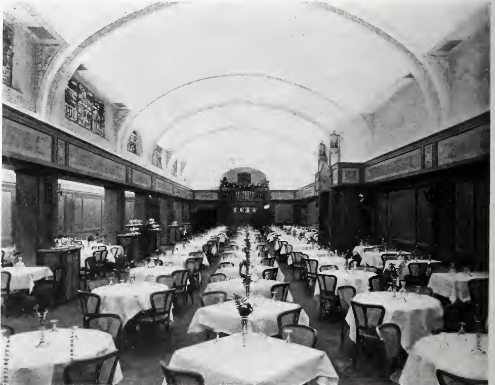
FIG. 14. A RESTAURANT INTERIOR SHOWING WELL DESIGNED COVE-LIGHTING. THIS IS MOST EFFECTIVE IF THE DESIGN OF THE ROOM DOES NOT PRODUCE AN IMPRESSION OF MONOTONY.
