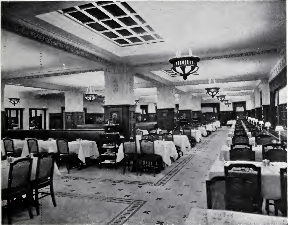
FIG. 15. A RESTAURANT INTERIOR IN WHICH INDIRECT LIGHTING HAS BEEN GIVEN DISTINCTION BY THE USE OF SPECIALLY DESIGNED FIXTURES.
