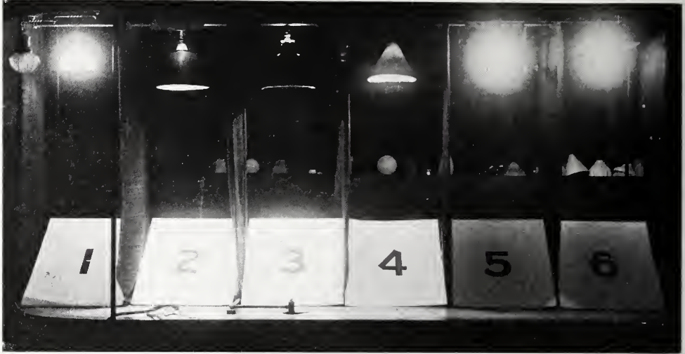
FIG. 7. A COMPARISON SHOWING THE EFFECTS OF VARIOUS REFLECTING SURFACES.
