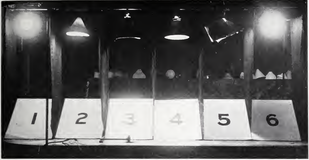
FIG. 8. COMPARISON OF WELSBACH REFLEX LAMPS WITH TUNGSTEN LAMPS, USING VARIOUS RE-DIRECTING AND TRANSMITTING MEDIA.
