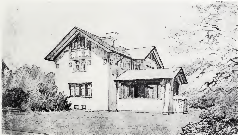
STUDY FOR A HOUSE ON A LEVEL SITE WITH FIRST FLOOR TWO FEET NINE INCHES ABOVE GRADE, AND UNBROKEN CONCRETE WATER-TABLE ON THE MASONRY WALLS OF THE BASEMENT. (See page 161.)
