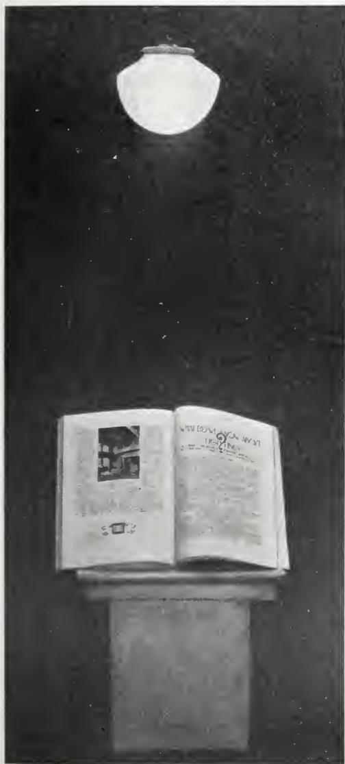
Photograph showing the modification of the distribution and increase of light below by the re-directive property of opal glass.
