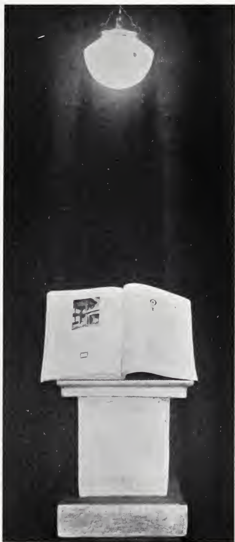
Photograph showing modification of distribution and loss of light below from a ground-glass globe.
