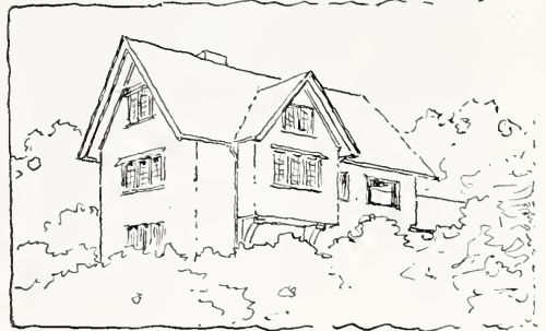
An awkward gable roof lacking preparation in the second floor plan for the cross-gable on the side, which is too large in proportion. The sketch shows a better treatment.
