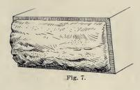
flat surface an inch or two in width, and much more smoothly wrought than the other parts. Thus, in Fig. 4 bis and in Fig. 7, the narrow band which surrounds the face is what is called a draft, and this draft is worked much smoother than the rest of the face. In the sketch before us it
