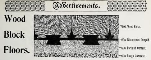
Composed of Wood Blocks cemented and keyed to a concrete foundation forming a solid and immovable structure, through which no dampness or foul air can penetrate and no disease germs or filth can be secreted. It is Fire-resisting, noiseless and warm to the feet, can be laid in a variety of patterns in different woods. Very handsome in appearance and everlasting.
