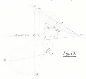
a vertical line from V  $P_a$ , putting one leg of the compass at V  $P_a$  and opening the other to J, this height can be swung around into the vertical position, thus locating the new V  $P_a$  where shown.
