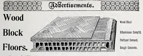
Composed of Wood Blocks cemented and keyed to a concrete foundation forming a solid and immovable structure, through which no dampness or foul air can penetrate and no disease germs or filth can be secreted. It is Fire-resisting, noiseless and warm to the feet, can be laid in a variety of patterns in different woods. Very handsome in appearance and everlasting.
