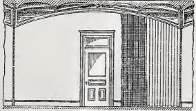
The PARTITIONS are solid, about two inches thick, formed of wire netting or metallic lathing and plaster.
