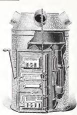
furnace is such that the heat impinges equally on all sides of the radiator, so that all the hotair pipes, if properly arranged, get an equal amount of heat, no one point being hotter than the other. One of the
