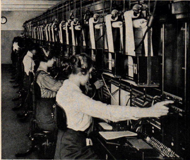
THIS TELEPHONE SWITCHBOARD IN ONE OF THE LARGEST HOTELS IN AMERICA IS COMPLETELY EQUIPPED WITH TELAUTOGRAPH INSTRUMENTS FOR EACH OPERATOR
