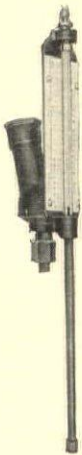
Hoffman Mercury Pressure Gauge. This gauge shows an exact reading in ounces of the pressure conditions at the boiler.
