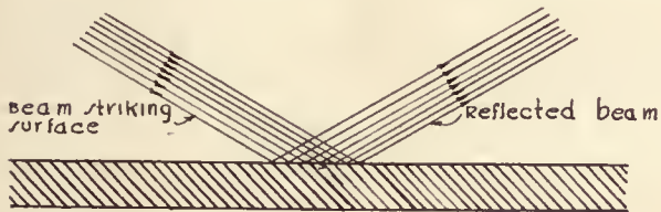
FIG. 1. REFLECTION. THE ANGLE OF INCIDENCE AND OF REFLECTION ARE EQUAL.
