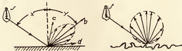
FIG. 4. AT LEFT: REFLECTION FROM SEMI-MAT SURFACE. AT RIGHT: REFLECTION FROM ROUGH MAT SURFACE
