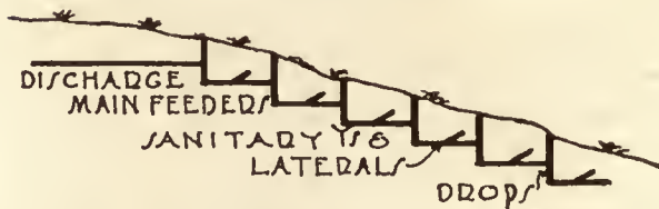
FIG. 2. THE STEPPED UP ARRANGEMENT OF THE MAIN FEEDERS HERE SHOWN IS NECESSARY WHEN THESE ARE LAID ON STEEPLY SLOPING GROUND
