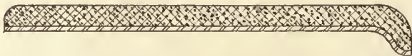
FIG. 17.—TREAD MADE OF ABRASIVE GRAINS IN LEAD MATRIX, THE WHOLE CARRIED ON STEEL PLATE, FLAT TOP
