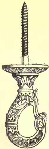
Fig. 421. Chandelier-hook with Catch. J. B. Johnston.
