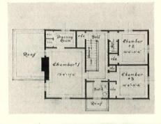
is faced with shiplap, the house is shingled and painted white, with dark green shutters and roof. Cubage, approximately 30,000 cu. ft.; cost, about 34 cents per cu. ft. Away from the New York area the architect has built similar work for 32 cents per cu. ft.
