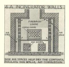
In laying out the incinerator, it is well for the architect to consult the manufacturer of several types, so that he may be well advised on the more essential points of the construction. The destructor should be large enough to take the accumulation of rubbish during at least one
