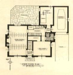
Roofing is of black asphalt shingles, excepting the roof over garage and laundry room, which is flat and is a built-up composition roof. Heat supplied by a warm-air furnace and an oil burner, the furnace being equipped with filters and automatic humidifier. Cubage, 17,800 feet, costing \$.278 per cubic foot
