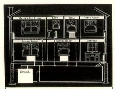
This shows you how simple the Burnham Unit-Air Conditioner System is. The Unit-Air Conditioners are located in the living and dining rooms downstairs and the master bedroom upstairs. Rest of heating done by the Burnham Slenderized Radiators.
