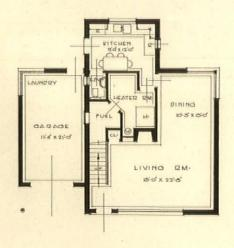
The house is built of cinder concrete block, with concrete joists and floor slabs. The concrete joists are exposed and painted. The house contains approximately 20,000 cubic feet, and the cost was \$.30 per cubic foot
