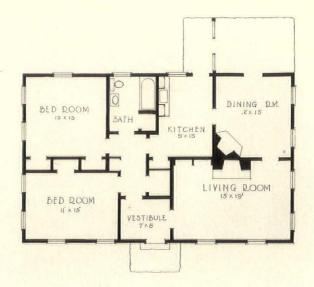
pine boards are used for flooring, treated with a dark stain filler and covered with dullsurface varnish. As to size, the house contains 17,835 cu. ft., and the cost was \$4000
