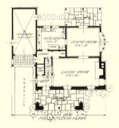
The house contains 27,900 cu ft., and cost \$8900, or about 32 cents per cu. ft. There is a full cellar under it. Front wall and porch are of Pennsylvania ledge stone, the other walls of frame construction covered by stucco and shingles. The roof is of slate, and is insulated. Inside, the baths are tiled, other floors oak, with the exception of linoleum in the kitchen
