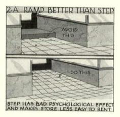
pled with the fact that this is more desirable from a psychological point of view, it reduces accidents. The material forming the ramp should have a non-slip substance in it so that even in wet weather there will be no danger of slipping. Where it is necessary, such as in high-priced locations, to have the store proper above or below the street level, access to this should be so arranged that there will be little feeling of going up or down steps.
