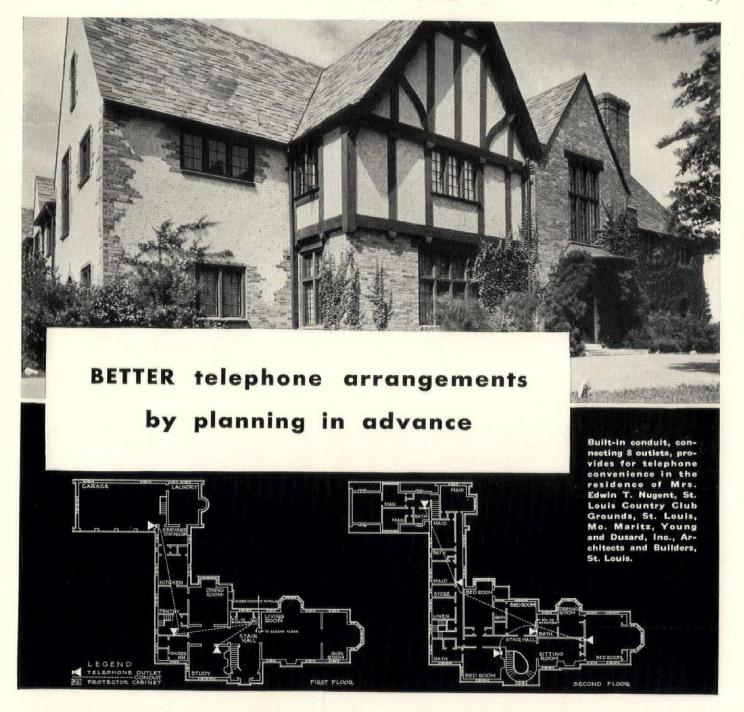
THERE are definite dollars-and-cents advantages to planning telephone arrangements as carefully as plumbing or lighting. Conduit, included in walls and floors during construction, costs very little — protects against certain types of service interruptions. Outlets located at convenient points permit telephones to be added at any time, easily, without exposed wiring.
