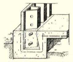
A perspective section showing a floor slab integral with footing for use at the first floor where there is no cellar
