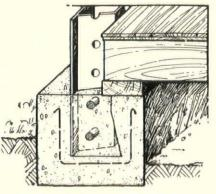
The F. K. unit for walls used in conjunction with wood floor joists and wood flooring. Note dowel bars and anchor slot into which steel is grouted
