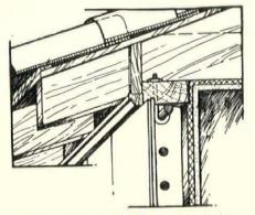
A perspective section illustrating the junction of wood rafters, ceiling joists, and plate over the Palmer cellular steel wall
