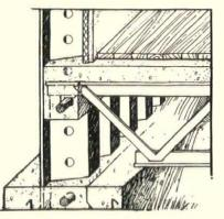
Standard construction of the single unit for walls with steel floor joists, concrete floor slab, and wood floor on mastic
