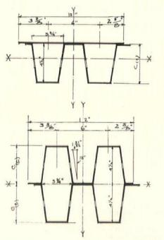
The flat keystone (F. K.) and the double keystone (D. K.) sections are typical designs for the steel load-bearing walls in the Palmer system. These copper-steel cellular sections are manufactured by the H. H. Robertson Co., of Pittsburgh, who have spent six years in the development of similar sections for floor use
