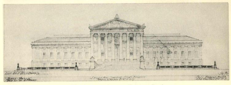
Three from among the many preliminary studies of the front elevation, in pencil on tracing paper. It will be noticed that on the upper one of these there was a flat dome provided in the composition. Each successive step in the study is marked by simplification and by the omission of decorative detail; the acroteria of the pediment, for example, disappeared before the building was erected
