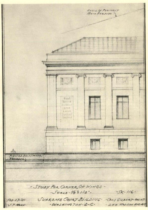
One of the preliminary studies for a corner of the wings. It was felt that the slope of the tile roof would approach closely the angle of the pediment in appearance when viewed from the street. Compare this with the photograph of the wing on the facing page
