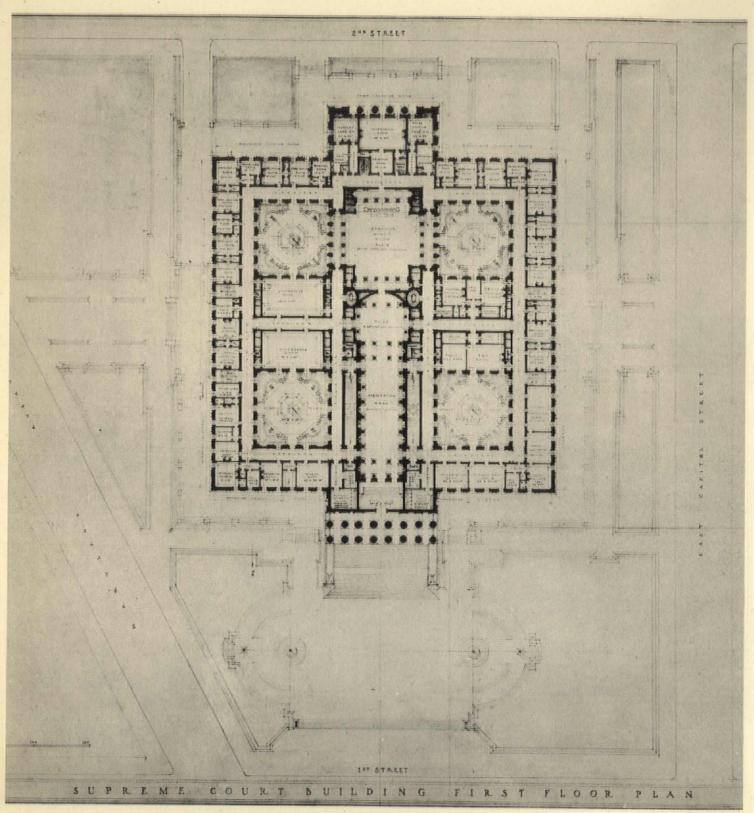
Plot plan and first floor. The east-west axis extending from First to Second Streets is a continuation of the axis of the entrance to the Senate wing of the Capitol. On the first-floor plan it will be noticed that the Supreme Court Room is the heart of the whole composition, flanked on either side by a courtyard and reached from the main entrance on First Street through the impressive Memorial Hall
