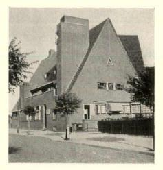
to the dominance of the steep roof. Note that the brick bond in the chimney differs from that in the walls. The flagpole, so often seen in Dutch work, is reached through a window at the top of a stairway in the chimney.
