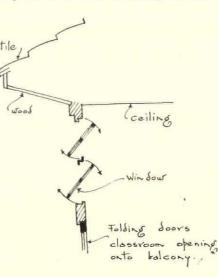
soffit is sloped up to the outside to gain more light indoors. The modern windows, pivoted horizontally, aid in weather protection while assuring ample ventilation.
