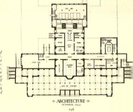
At right, plan of the basement floor. At the top of the plan is the location of the ovens. Elevators lower the bodies from the large and the small halls to space beneath, from which they are wheeled to the ovens
