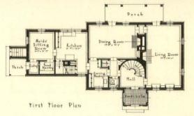
Plan of the first floor. In spite of the comparatively small size of the house, its plan is given real distinction with the semicircular stairway
