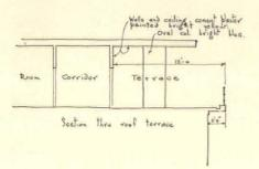
its projection is included in the 12' required for the firemen, and these worthies, it is hoped will not often have to use the partly covered terrace that the setback affords. The large oval column shown in the section carries all piping for these Mount Royal Flats to the roof, from which gravity flow is employed to reach the rooms.
