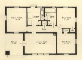
with little obsolescence and small maintenance cost. The first floor is a concrete slab on a sand fill, covered with asphalt tile. Secondary partitions are solid plaster on metal lath and steel studs
