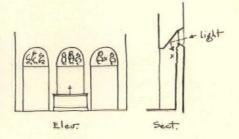
the reredos. The source of light, as the diagram shows, is invisible from inside the church.
