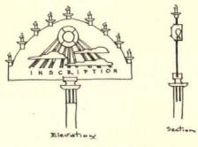
The sun's rays are of sheet iron, gilded and fastened to the main plate. Clouds are of black iron put on over the rays. The sun itself is opal glass with a light behind it.
