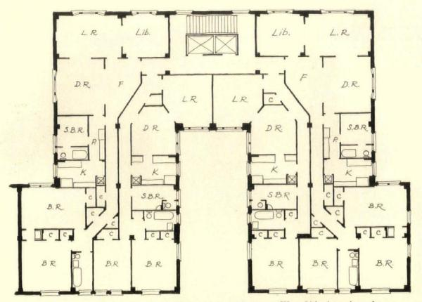
Here is one of the better elevator apartments on the upper West Side, its suites of seven, eight, and nine rooms once in great demand. Its modernization necessitated practically the entire rebuilding of the interior, with the typical floor divided as below. Voorhees, Gmelin & Walker were the architects
