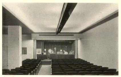
A conference room in the General Electric Company Building, New York City—Hood & Fouilhoux, architects. The trough fixture running down the middle of the ceiling is that shown in detail on the previous page. In a gun-metal mirror trough the neon and mercury vapor lamps produce a visually white light as well as varied color combinations. The scheme was conceived by A. L. Powell, illuminating engineer, and executed by the A. Ward Hendrickson Co., Inc.
