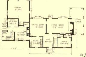
Below are the plans of the first and second floors. An attic stairway provides for two bedrooms and a bath above, when future expansion is desirable
