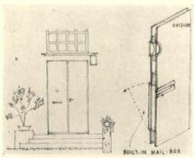
tred above its slot is a peep hole. The construction of both of these accessories is shown in the section.
