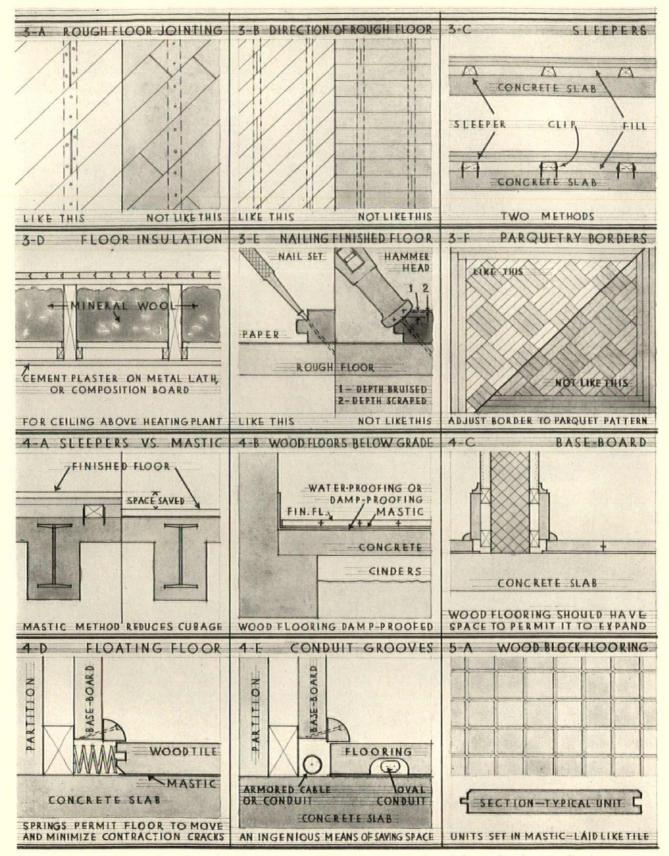
Remember that the life of the finished floor will be no longer than that of the under-floor or the sleepers; provide for insulation where needed; watch out for the "nailing butcher," the relation of borders to parquetry; consider the advantages of mastic; check your damp-proofing, provision for expansion and wiring conduits, and any processed wood flooring
