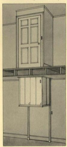
only an opening, cab size, between first and second floors; above, is enclosed in its own closet. Standard model, 30" x 30" platform, lift of over 350 pounds. Special model, 36" x 36". The Shepard Elevator Co., Inc., 2413 Colerain Avenue, Cincinnati, Ohio. 321
