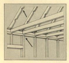
product, constant as to size and shape, 75 per cent of which is pre-cut ready to place. Does not limit architectural expression. Framing members go together with Enterlock (patented) wedge-shaped dovetailed joint. Long-Bell Lumber Sales Corp., Kansas City, Mo. 47
