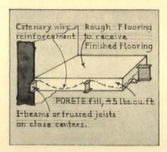
centres, resulting in a lightweight fireproof floor with flat ceiling and excellent sound and heat insulation. Can be erected by any contractor under Porete Company supervision. Porete Mfg. Co., North Arlington, N. J.
