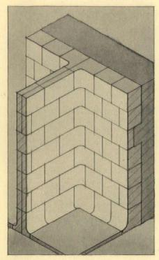
either gloss or eggshell ceramic surface. For face size of 8" x 4¾" there are three thicknesses: 3½" for load-bearing, 3" for wainscot, 1½" for light veneering. Machine-ground to accurate size and angles. Colors: white, black, twenty-five pastel shades; gloss, eggshell, or textured. Usual line of shapes. American Enameled Brick Corp., Graybar Bldg., New York, N. Y.
