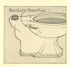
struction of bowl, rather than any mechanical device, holds the water level in the bowl below the flushing rim, preventing cross connection and therefore back siphonage. The John Douglas Co., Cincinnati, Ohio.
