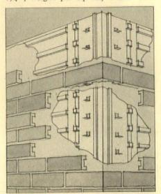
covered with waterproof building paper; nail on the special steel field sheets and corner sheets; apply waterproof cement mortar; key on the lock brick. Tub-Hill, Inc., Pittsburgh, Pa.
