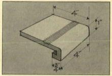
tile line. Nosing itself almost square, so that end return fits well into wall designs. Non-slip ribs project 31" above face. The Sparta Ceramic Co., 110 E. 42d Street, New York, N. Y. 70
