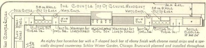
An eighty foot horseshoe bar with a T-shaped back bar of ebony finish with chrome metal strips and a specially designed counterstep. Schlitz Winter Garden, Chicago. Brunswick planned and installed throughout.
