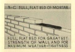
a little mortar between the spaces. The joints around the chimney are especially vulnerable points and should not be neglected. Particularly is this so of the space between the flue lining and the brickwork. This space should be absolutely tight. All firebrick will, of course, be called for to be laid in fire clay. Joints between flue pipes should be struck.
