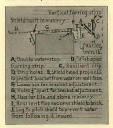
space of 2", but is adjustable for any depth required. Metal sleeve built in masonry, adjustable bracket arm and V-shaped horizontal furring strips clipped to arm. Simplon Products Corp., 551 Fifth Avenue, New York, N. Y.
