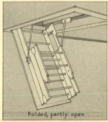
panel within ceiling opening. Straight coil springs hold balance in any position. Panel size, 28" x 60", for ceiling heights up to 9' 10". (Model 66 for heights up to 12'.) The Marschke Co., 551 University Avenue, St. Paul, Minn.
