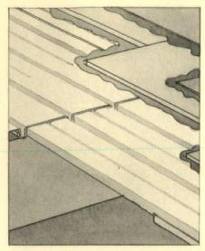
steel, 18" wide, also in 6" and 12" widths. Covered merely by insulation and waterproofing. Sold erected in place. United States Gypsum Co., Chicago, Ill.
