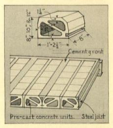
between the blocks, resulting in a light floor with flat ceiling. Columbia University tests show this floor to resist a four-hour fire. Porete Mfg. Co., North Arlington, N. J.
