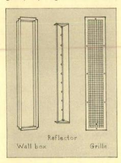
porcelain-enamelled in colors. Reflector of chromium-plated steel. Wall box of steel, black enamelled, with knockouts. For 115 volts, 1650 watts; for 230 volts, 1650 and 2000 watts. Thermador Electrical Mfg. Co., 116 Llewellyn Street, Los Angeles, Calif.
