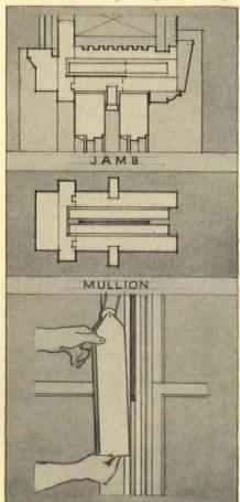
with pulley replaces two ordinary weights. Bronze weatherstripping is standard equipment. A special "Heavy Duty Narroline" is also made for large windows. Andersen Frame Corp., Bayport, Minn. 48
