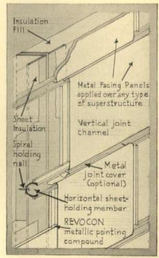
pound provides a weather-proof joint. Insulation can be attached to rear. Glass can be fitted snugly. Aluminum Co. of America, Pittsburgh, Pa. 34
