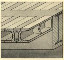
6' (also 4' and 5'), reinforced to carry temporary floor loads before T-beam is poured. Spans 10' to 25'; floor loads, 40–125 pounds per square foot. Porete Mfg. Co., North Arlington, N. J. 8
