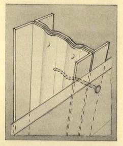
tural design. Erected by carpenters. Permits nailing collateral material directly to steel. Fire-safe, will not warp, termite-proof, salvageable. Stran-Steel Corp., Detroit, Mich.
