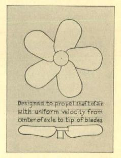
blades diminishes toward the tips. This means a smaller propeller, slower speed, smaller motor. Frames are one-piece cast aluminum. The Allen Corporation, 14th Avenue at Howard Street, Detroit, Mich.
