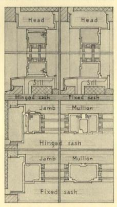
floor, and glazed with structural glass at floor-level spandrels. Any combination of single and double glazing, with operating or fixed sash. The Kawneer Co., Niles, Mich.
