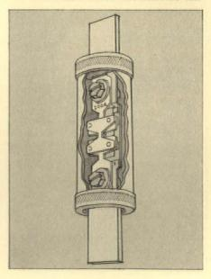
perage of fuse, but the attached lagplates give greater heat capacity and slow down blowing time, giving harmless overloads a chance to clear. Protection is not sacrificed. Prevents needless shut-downs. Bussman Mfg. Co., University at Jefferson, St. Louis, Mo. 243
