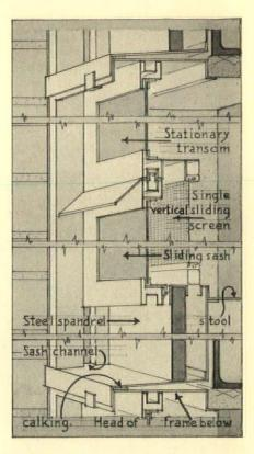
down back of spandrel, sash that slide down over spandrel. Sash operated without opening screen. Window washing done from inside the room. Corry-Jamestown Mfg. Corp., Corry, Pa. 46
