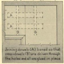
is built in under pressure, the pins locked through the dowels. Panels of Harbord plywood. Harbord Plywood Corp., Hoquiam, Wash.
