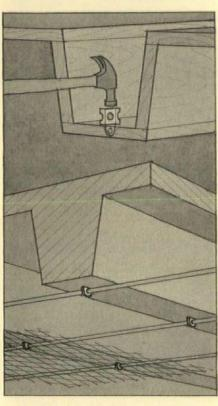
moved the driven blade with hole is exposed to which to fasten wire or 1/4" (also 1/6" size) rod. Permits flat lath instead of high-rib. Union Steel Products Co., Albion, Mich.
