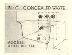
ports the tub on the studs and permits of easy levelling. On floors other than wood the tubs should be well set on bricks or cement blocks. This will prevent strains or cracks between tub and tile, caused either from settling, or by unusually heavy
