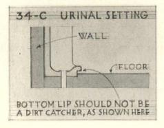
suggested that a note be put in floor tiling specifications calling for the floor to be slightly pitched to the urinal, if the floor type is used, and slightly away from it if either the pedestal or wall-hung type is used. If installed in public places it might be well to consider a treadle type instead of a button-operated valve, which seldom works and few care to touch.
