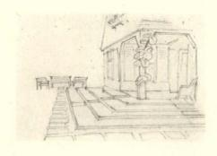
L'ARCHITETTURA ITALI-ANA illustrates an ingenious inn for overnight tourist business, designed by Vittorio Bonade-Bottino. It is a tower constructed of reinforced concrete in which the rooms open from a spirally ascending ramp. It will be noticed from the exterior that the horizontal line of windows follows this same spiral, at a slope gradual enough to be almost un-
