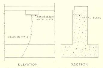
The above drawings illustrate a simple method of blocking the passage of termites through a crack in the foundation wall. A hole is cut through the wall above the crack, a metal plate set in a bed of rich cement mortar, and the hole packed solid with a mixture of rather dry cement mortar.
