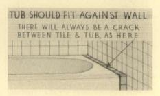
ing a band of split tile to be run between the tub and the wall. The architect should ask for, and get, the roughing size of the tub. This will enable him to do his part in laying out a workmanlike job of the bathroom.
