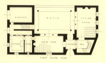
patio. The house is of adobe construction. The plan differs somewhat from the finished work in that the outside wall of the patio was closed up to the level of the second-floor gallery, and a door from the garage opens into the patio
