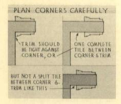
danger that the door may be moved too far over to the one side, with the result that only a small strip of tile is possible, or that the trim of the door must be cut. Both of the latter are undesirable features that can be avoided.
