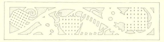
In order that no screws, rivets, or other means of attachment might show upon the face of the work, it was determined to fasten the laminations together with pins fixed to the back of each piece. Therefore, the templates were spotted for the pins and for the holes to match them, drilled and fitted together. Then, the locations of pins and holes were transferred to the plates with a center-punch. The pins, of a non-ferrous metal, were brazed to the backs of
