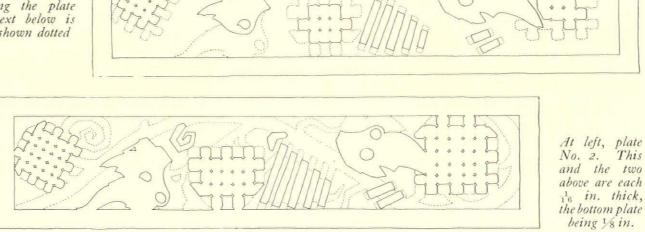
At right, plate No. 1, next to the wood. The perforations are shown stippled
