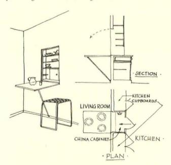
work of Gottfried Schramm, an architect of Hamburg. *Moderne Bauformen* shows this folding dining-table which drops down into the living-room, and is served through the opening in the thickness of the kitchen cupboards from the kitchen itself.
