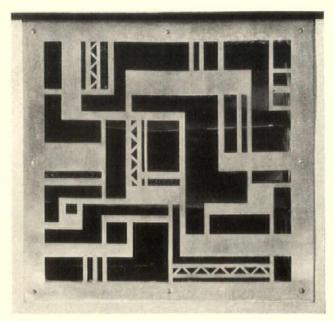
Both the grilles above have been stamped from a single sheet of monel metal. While the patterns are not structural, they are satisfactory because they are relatively small and no great strength is necessary. In metal work such as this it is to be hoped that designers will appreciate the limitations of non-structural forms, avoiding them where strength is essential to satisfy the eye. Ross&MacDonald, architects; Sproat Rolph, associated. Craftsmanship by The Architectural Pronze and Iron Works
