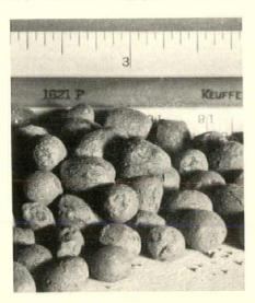
face shell, while the firm interior is filled with air cells. Concrete made from this new product, with natural sand for the fine aggregate, is said to possess a most unusual combination of workability, strength, and light weight, together with highly efficient insulating qualities. W. F. MacGlashan Associates, Alhambra, Calif.
