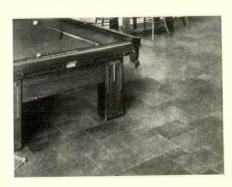
of t. & g. construction providing interlocking joints. Squares, 6", 9", and 12"; borders, 3", 6", and 12" wide and 47" long. Surface of Presdwood resists wear and shows no indentations. Masonite Corporation, Chicago.
