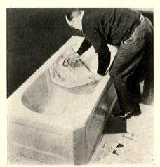
Applied with common paint brush. Hard covering that withstands all common abuses. Removed by soaking with water and peeling off. Kohler Company, Kohler, Wis.
