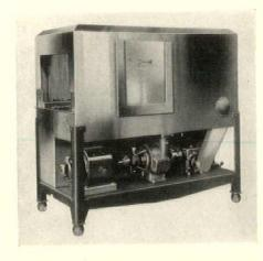
The new type Colt Autosan pump, fitted with special front plates to make possible inside inspection and cleaning. 2. A new type of spray arm, radically different in inside design from the standard type of spray arm and operating on an "intercepting" principle. 3. Every possible bend has been eliminated from manifold and feed lines, cutting down resistance and increasing power. Colt Patent Fire Arms Mfg. Company, Hartford, Conn.
