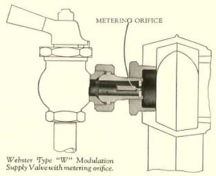
can enter is correspondingly restricted. As a result the steam soon flows on through the piping to the next radiator where the restriction of the orifice is slightly less, because the pressure of the steam as it reaches this further point is lower. So it goes, radiator by radiator, to the furthest point—the "pressure drop" to each radiator being equalized or balanced by installation of properly sized metering orifices.
