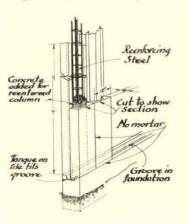
Here is an isometric drawing of a foundation with tiles in place.
