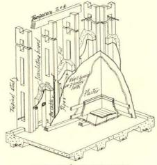
ISOMETRIC VIEW Shampy PRECAST STUDS IN WALL
