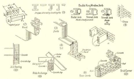
In the upper left corner are shown the dimensions of the unit and the several diagrams illustrate various details of construction with its use
