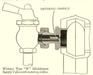
flow in accordance with the need for steam at every point of radiation . . . Thus all radiators get steam at the same time and in substantially the same proportion. No overheated rooms, no cold spots.
