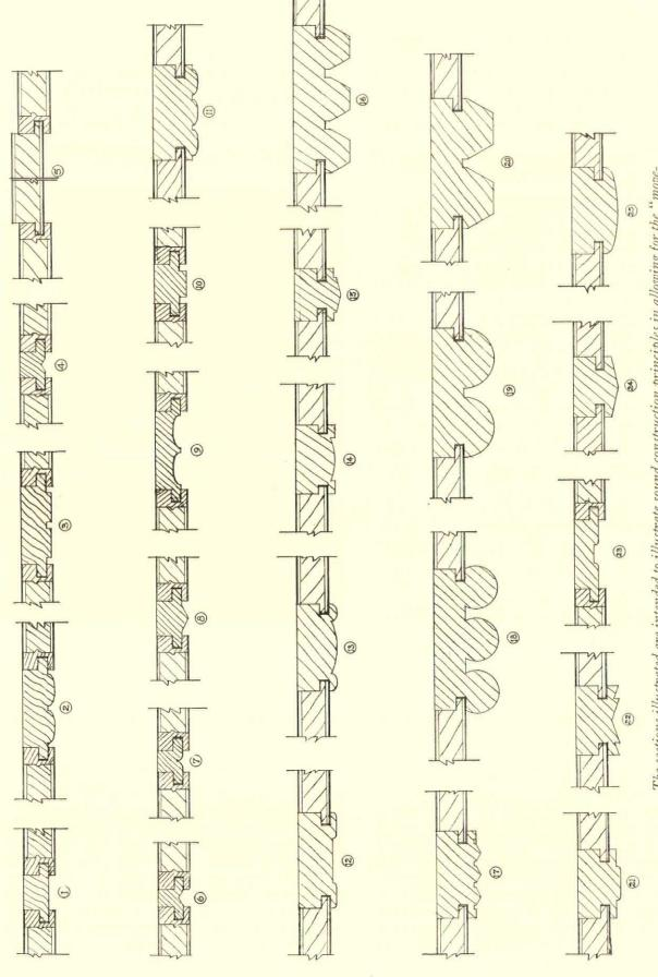
The sections illustrated are intended to illustrate sound construction principles in allowing for the "movement," of woodwork; they are not offered as suggestions in decorative design. These inserts should be spaced not less than six or seven feet apart in veneered plywood, and they may be of the same wood as the panels, or of a contrasting wood, or of metal
