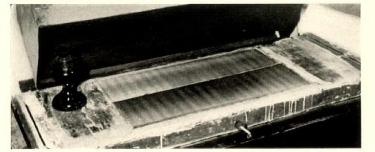
Here is the apparatus used in Dr. Hooper's tests—a section of plastered wall and a metal box in which soot could rapidly be produced. The two sections of plaster shown here were separated by a partition underneath, separating cold air and warm air currents. The lath marks in the former are between the laths; in the latter, over the laths
