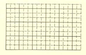
Fig. 1. Corner of ruled sheet for working drawings; each large square represents 3 feet 9 inches at eighth scale
