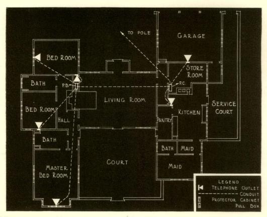
Complete telephone convenience is provided in the residence of Dr. George W. Hawley, Bridgeport, Connecticut, by six telephone outlets, including one in the garage. The telephone wiring is carried in conduit bidden in the walls and floors. FRED C. JOHNSON, Architect, Bridgeport.
