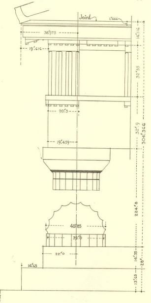
FIG. 3. Temple of Theseus: Detail of the Order, from Stuart and Revett, with figures in inches
