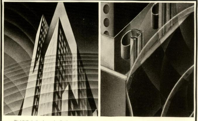
The left illustration shows noise vibrations crashing against the exterior of a building, like waves breaking on the seashore. At the right is a USG sound insulated "floating" partition which prevents similar sounds created within the building from being transmitted from one room to another.
