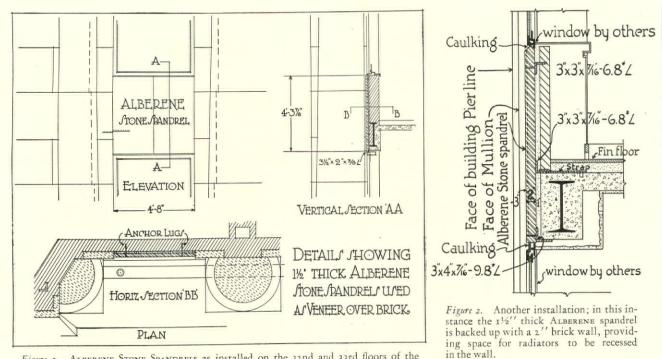
Figure 1. Alberene Stone Spandrels as installed on the 32nd and 33rd floors of the Newark & Essex Bank Building
