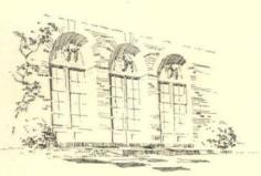
Not infrequently in residential work three arches have French doors in the centre, flanked by double-hung sash. When 3/4"-scale details are made it becomes evident that, unless the stiles of the doors are cut down to 21/2" to 3" in width, the amount of wood showing at the head rail will differ widely between the doors and windows. From a design standpoint the three openings should appear alike.
